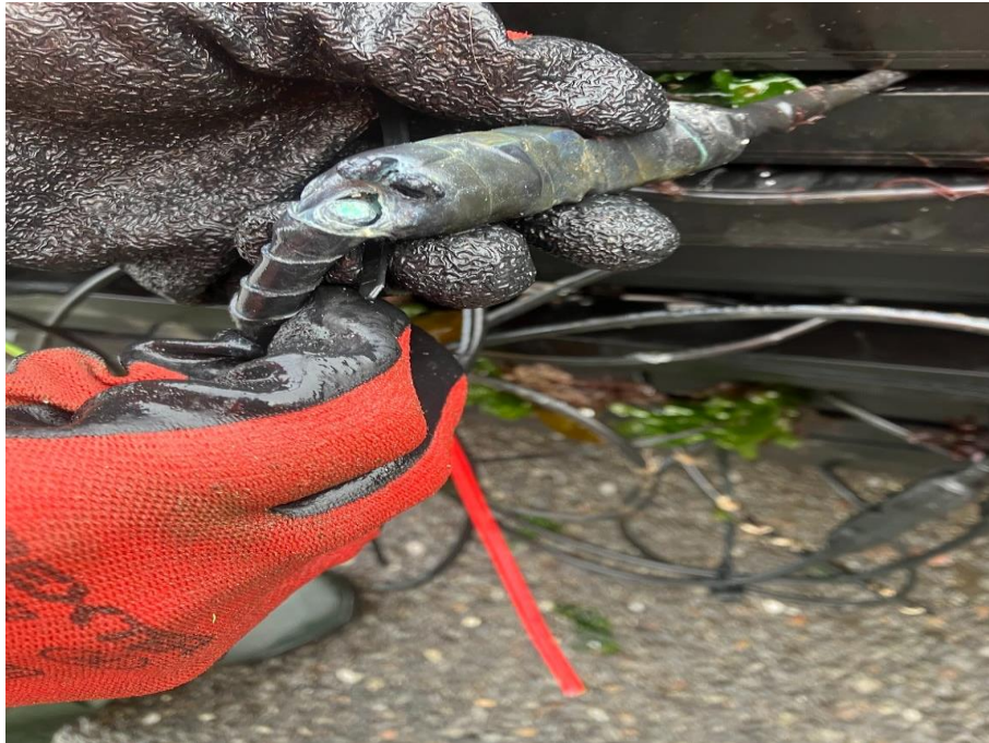
Figure 11. Corrosion damage to a standard MC4 connector exposed to saline marine conditions, showing copper oxidation (“green rot”) and insulation degradation caused by salt aerosol ingress, thermal cycling, and DC-induced electrochemical reactions.
