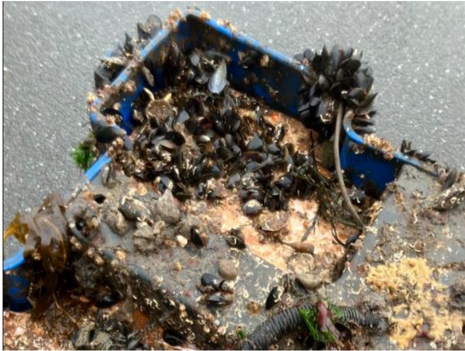
Figure 13. Biofouling of a submerged floater, showing extensive mussel colonization and marine growth leading to increased structural mass, reduced buoyancy reserve, and restricted movement of articulated components.
